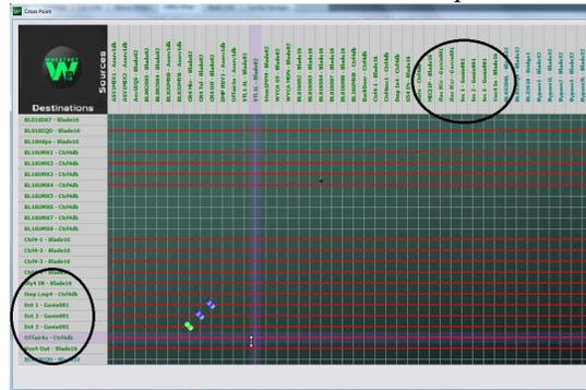
**This is the WheatNet Navigator crosspoint screen showing the crosspoint connections for the Genie. Look Ma! No wires!**
