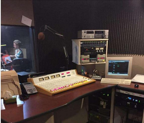
**Figure 2 - The crew wanted an older board with analog meters. We temporarily dropped in an R60 from storage.**
