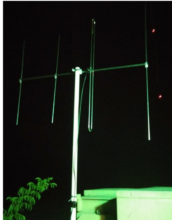
Figure 4 - Temporary mount using hose clamps and tape, but it works!
