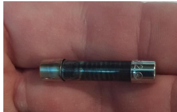
Figure 3 - What a thoroughly blowed-up fuse might look like.
