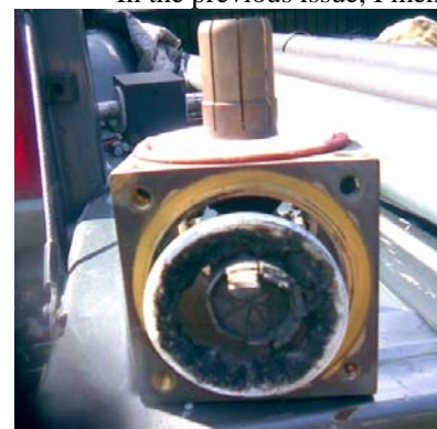
A burned-out bullet produced damage below the joint
