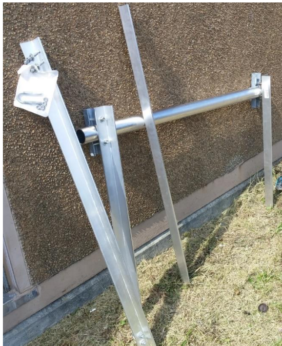
Figure 1 - Left, the bracket for the lowered unipole "skirt" wire; right, the bracket, ready for drilling and final cuts.
