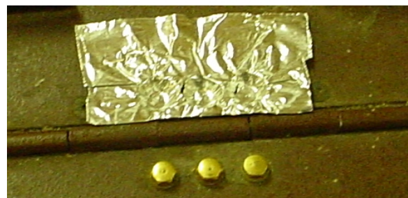
The "fix" for leakage into the FIM
