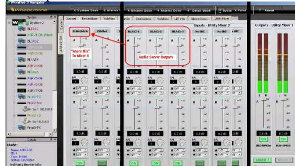
Figure 2 - We use Mixer Y to make the audio server mix, then assign all sources as they were on our old ACU1s.
