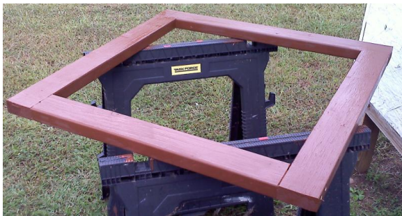
Figure 1 - Wooden frame, treated with weatherproof stain
