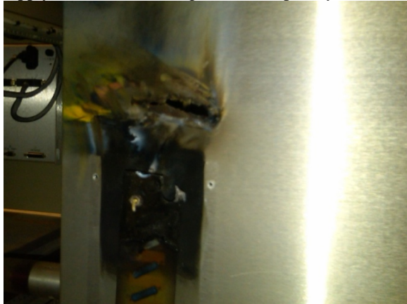
Figure 1 – The arc burned a gash through the FM-30T cavity wall
