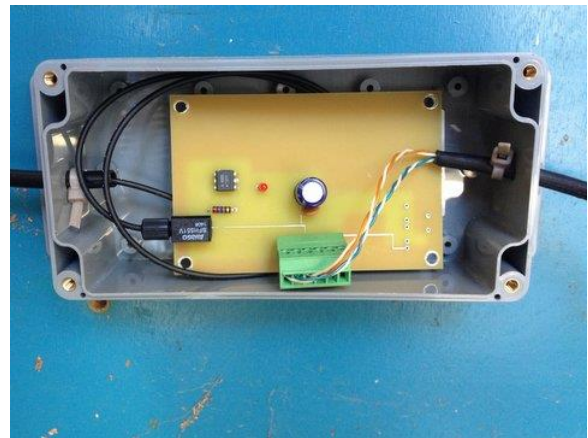
Fiber-optic receiver board mounted in a weatherproof box inside the tuning house. The fiber enters at the lower left.
