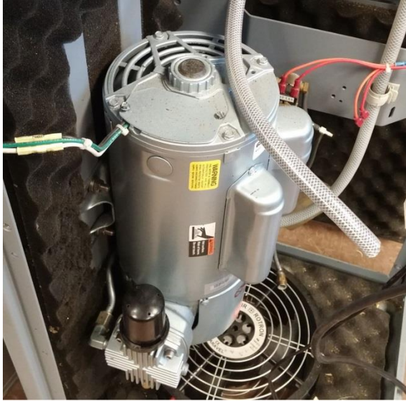
Figure 3 - The rebuilt compressor, ready to be rewired and moved back to Cullman.
