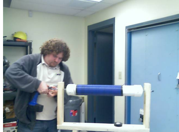
Jimmy prepares the choke to receive two more windings.
