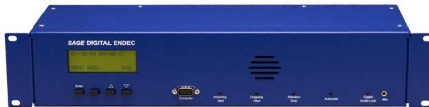
installation where an AES feed is taken from the unit). “Simulcast” must be enabled for the digital output to work. This was not clear in the manual, which seemed to indicate that if the digital output was enabled you would be good to go. We quickly found that the relay would generate a program interrupt in the bridge but no header/message/EOM would be transmitted. Enabling “simulcast” fixed that.
