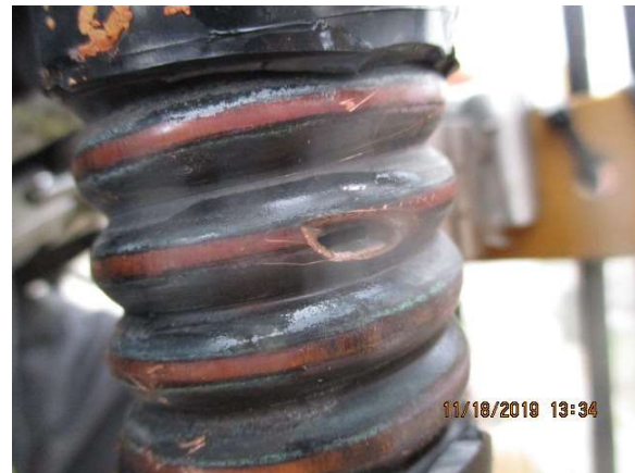
A broken butterfly clip rubbed this hole in the line.
