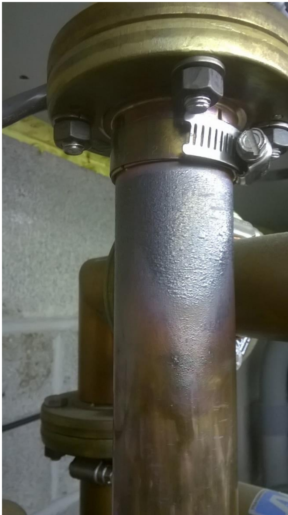
The burn was apparent on the outside of the line section.
