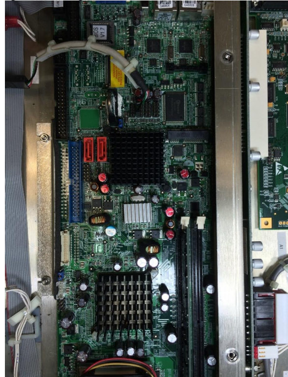
The capacitors marked in red in this photo are the ones that should be replaced on the Nautel Exporter Plus SBC.
