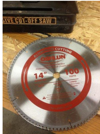
A 14" 100-tooth non-ferrous blade is perfect for cutting tubing and transmission line.
