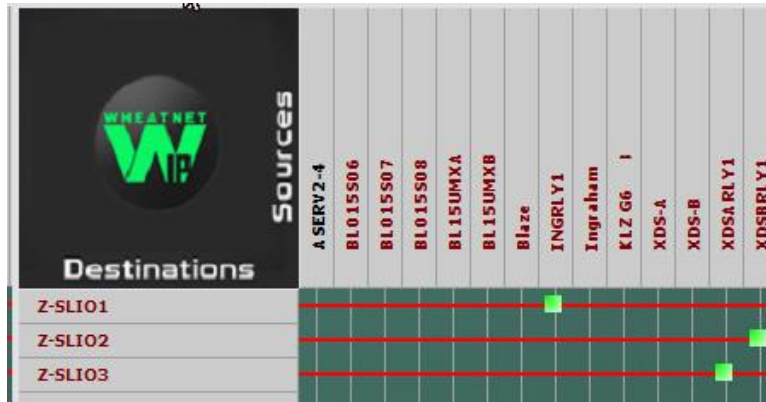
Figure 2 - KLZ crosspoints showing logic input sources mapped to soft logic output destinations for satellite relays
