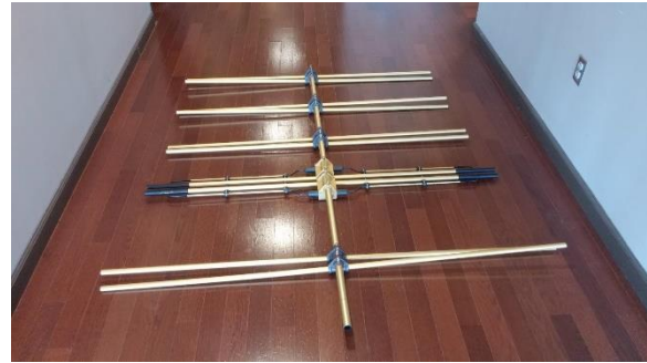
Figure 2 - The Scala Yagi cross-polarized antenna being assembled.
