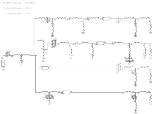
**Figure 1 - Nodal Circuit Model of the KBRT Antenna System**
