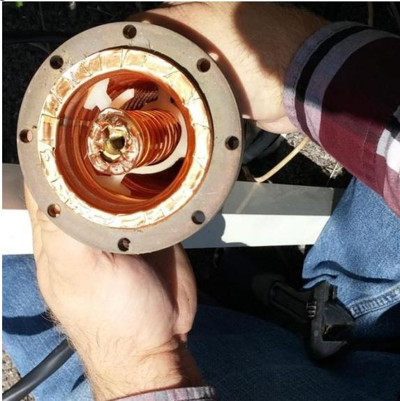
**Figure 2 - Tower #5 at WXJC. Note the gap between the inner conductor and the screw connector.**
