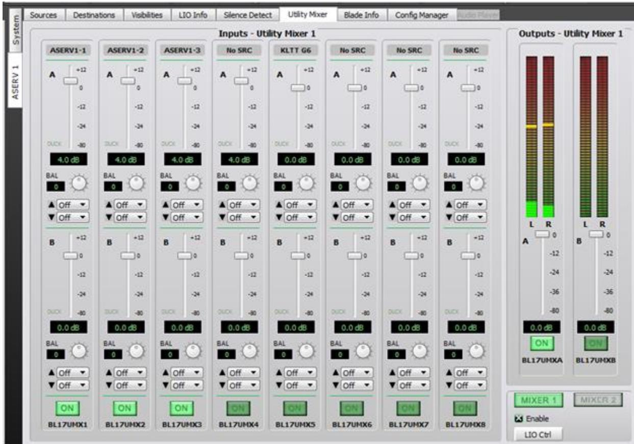
**ASERV Blade Utility Mixer Configured for Control Room Bypass (ASERV Direct to Air)**
