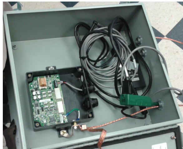
Figure 2 - Sealed NEMA box for the power supplies
